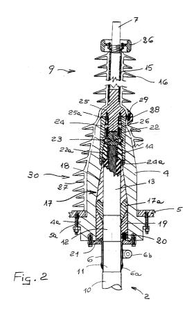
The present invention relates to a terminal for an electric cable, in particular to a terminal for a medium and high-voltage electric cable for external use, that is adapted to be used outdoors, being exposed to the air and possible polluting agents.
