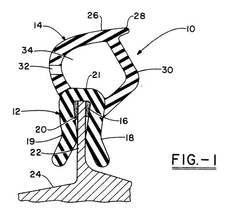
This specification relates to weatherstrip profiles. In particular aspects it relates to sealing weatherstrip profiles useful for sealing moveable components, especially for sealing moveable closures furnished as coverings for openings providing access to regions of automobiles, trucks, and other vehicles. In preferred aspects it relates to weatherstrip profiles that do not require reinforcement, particularly metal reinforcement, to secure them to flanges.
