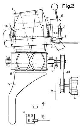
The present invention relates to a method for removing the end of coils externally wound onto the side of a basically flat-tapered bobbin in formation.
