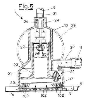
The present invention relates to a pneumatic sensor for a safety device for blocking the water feed circuit of dishwashers, washing machines and the like
