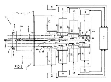
The present invention relates to a process for controlling the horizontal movements of yarn carrier bars, correlated with a predetermined distance between centres of the knitting needles in knitting machines, comprising the use of a plurality of stepping motors each operatively connected to a yarn carrier bar for transmitting reciprocating movements having variable-width strokes to said bar, as wall as a central control unit managing working cycles carried out by said stepping motors.
