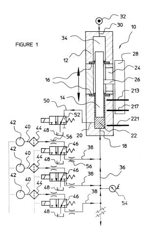
The present invention relates to volumetric metering equipment, especially but not exclusively for use in metering the volume of fluid pumped through one or more injectors by a diesel-engine fuel injection pump.
