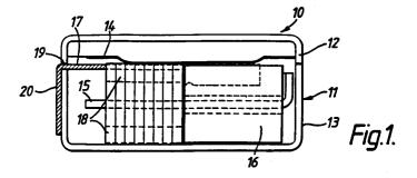
This invention relates to electrical coil assemblies and in particular, but not exclusively, to such assemblies for use in hearing aid transducers.
