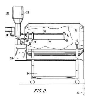
The invention relates to an apparatus for application of powdered or granular material on a solid product. In particular, the invention relates to the application of a seasoning or spice on a snack food such as potato chips, corn chips or the like.
