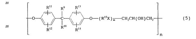
wherein R<sup>9</sup> - R<sup>14</sup> may be the same or different and are hydrogen or an alkyl group of 1 to 3 carbon atoms, R<sup>15</sup> is an alkylene group of 2 to 5 carbon atoms, X is an ether or ester group, m is an integer of 0 to 3 and n is an integer of 20 to 300,
