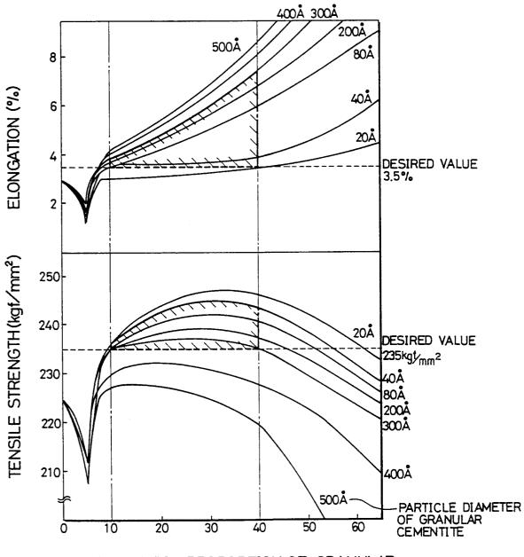
VOLUMETRIC PROPORTION OF GRANULAR CEMENTITE TO THE TOTAL CEMENTITE AFTER THE HEAT TREATMENT (%)
