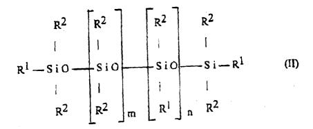
wherein R<sup>2</sup> is independently selected from hydrocarbon or halogenated hydrocarbon groups having 1 to 10 carbon atoms. R<sup>1</sup> is independently selected from R<sup>2</sup> or a eugenol residue. m is an integer having an average value of 5 to 500 and n is an integer having an average value of 0 to 500. with the proviso that there is at least one eugenol residue in the molecule. Also disclosed is a composition comprising an organopolysiloxane and the above heat-resistant agent.
