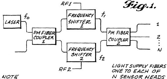
FIBERS HERE ARE POLARIZATION - MAINTAINING (PM)
