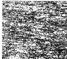
The composition has a transformation start temperature ( $B_s$ ) of  $670^{\circ}\text{C}$  or less. Since the steel product obtained by the method has no variation in physical properties regardless of variation in cooling rate, it is possible to supply steel products of high strength and high toughness which have uniform microstructure and properties along their thickness direction and are excellent in weldability.
