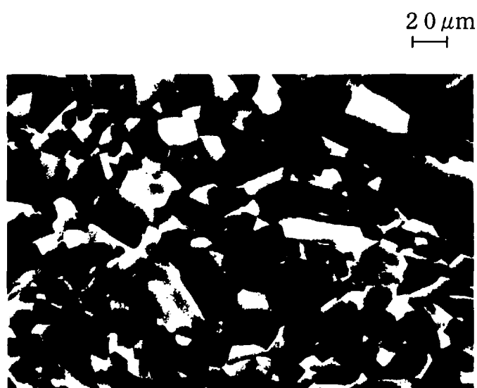
No. 4 (Average grain size 9μm; comparative sample)
