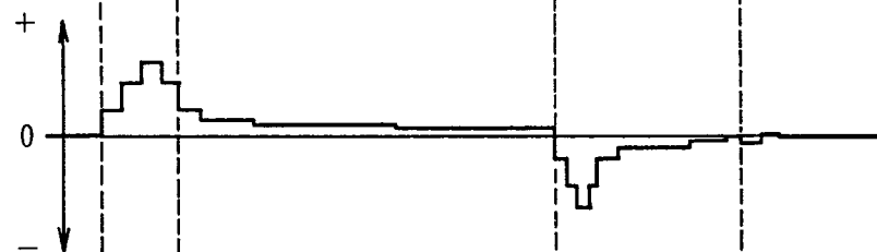
FIG. 16C LENS ACTUATOR CURRENT I_a
