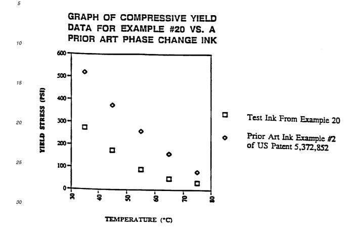
Tests were done on an MTS SINTECH 2/D mechanical tester using cylindrical sample blocks about 19mmx19mm.
