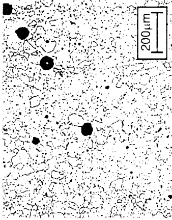
ASTM 6.5 Grain Size / 2.1% Porosity
