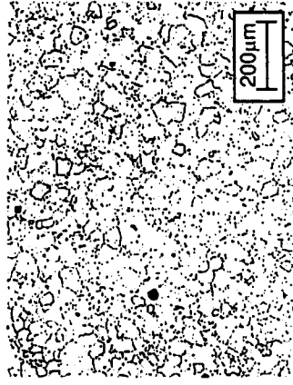
ASTM 6.5 Grain Size / 0.9% Porosity
