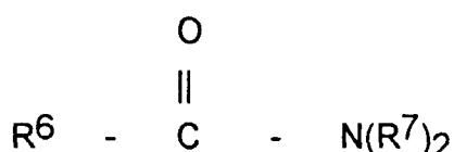
wherein  $R^6$  is an alkyl group containing from 7 to 21, preferably from 9 to 17, carbon atoms and each  $R^7$  is selected from the group consisting of hydrogen,  $C_1$ - $C_4$  alkyl,  $C_1$ - $C_4$  hydroxyalkyl, and  $-(C_2H_4O)_xH$  where  $x$  varies from 1 to about 3.
