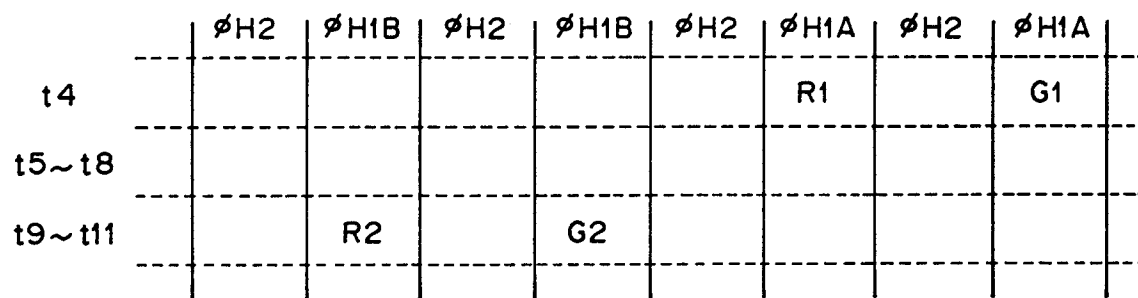
HORIZONTAL TRANSFER REGISTER CHARGE TRANSFER DIAGRAM
