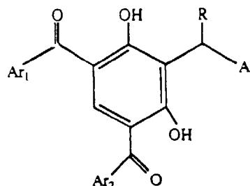
10 in which Ar<sub>1</sub> and Ar<sub>2</sub> are independently substituted or unsubstituted monocyclic or polycyclic aryl groups, R is hydrogen or an aliphatic group of from 1 to 8 carbons and A is an oxirane (epoxide) group. The oxirane can be ring opened to provide derivatives as described herein.
