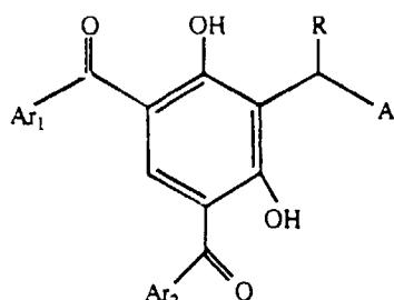
where  $Ar_1$  and  $Ar_2$  are independently substituted or unsubstituted monocyclic or polycyclic aryl groups, R is hydrogen, or an aliphatic group having from 1 to 8 carbon atoms, and A is an epoxy or a ring-opened residue of the epoxy group.
