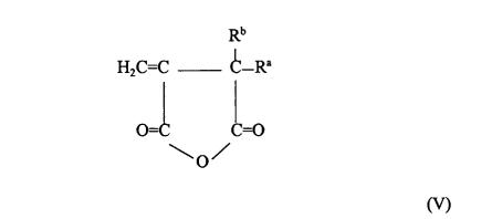
wherein R<sup>a</sup> and R<sup>b</sup> independently represent hydrogen or an alkyl group having 1 to 4 carbon atoms. Specific examples of monomers C include itaconic anhydride, citraconic anhydride and maleic anhydride. Maleic anhydride is especially preferred.
