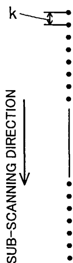
Fig. 5 (B) DOTS FORMED BY ONE NOZZLE ARRAY
