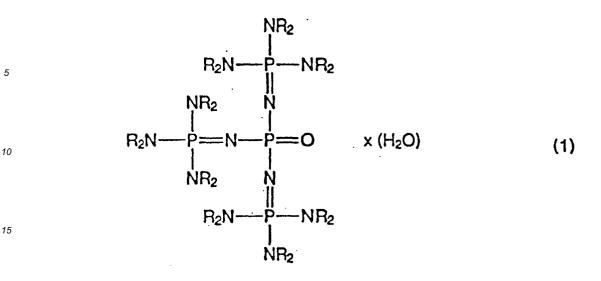
wherein each R is the same or different and each represents a hydrocarbon group having 1 to 10 carbon atoms, and x is within a range from 0 to 5.0,
