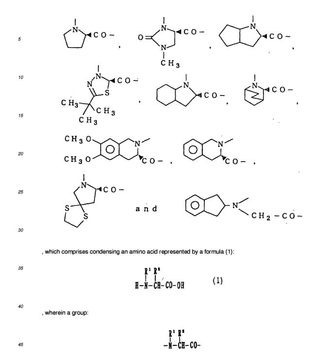
is the same as defined above, and N-(1(S)-ethoxycarbonyl-3-phenylpropyl)-L-alanine • N-carboxyanhydride under basic condition, decarboxylating a produced carbamic acid derivative under between neutral and acidic condition to obtain an N-(1(S)-ethoxycarbonyl-3-phenylpropyl)-L-alanyl-amino acid (2), and forming a pharmacologically acceptable salt thereof,
