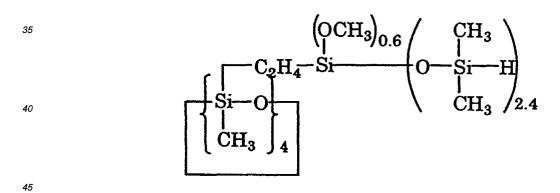
6. The heat-curable silicone rubber composition of Claim 1 where the carbosiloxane dendrimer is selected from the group consisting essentially of carbosiloxane dendrimers having the following general formulas
