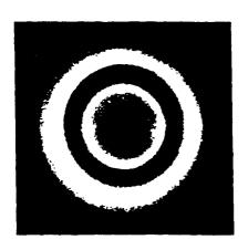
X-ray diffraction image of  $\beta$ -type silk fibroin
