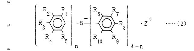
(wherein  $R_1$ ,  $R_2$ ,  $R_3$ ,  $R_4$ ,  $R_5$ ,  $R_6$ ,  $R_7$ ,  $R_8$ ,  $R_9$  and  $R_{10}$  independently represent a hydrogen atom, a fluorine atom, a hydrocarbon group or an alkoxy group, at least one of  $R_1$  to  $R_5$  is a fluorine atom, at least one of  $R_6$  to  $R_{10}$  is a fluorine atom,  $Z^+$  is a monovalent cation seed, and n is 3 or 4).
