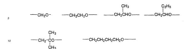
The main chain skeleton of the polyoxyalkylene polymer may consist of either one or two or more repeating units. In case of a curable resin composition to be used as, for example, a sealant, it is preferable to employ a polymer having oxypropylene as the main component.
