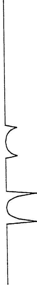
F i g. 6E EMITTER VOLTAGE OF TRANSISTORS 34 ( IMAGE QUALITY CORRECTION SIGNAL )
