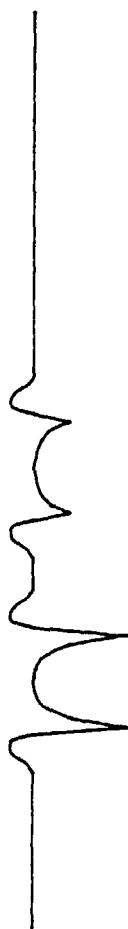
Fig. 7E EMITTER VOLTAGE OF TRANSISTORS 34 (IMAGE QUALITY CORRECTION SIGNAL)
