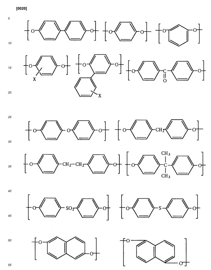
**[0021]** The liquid crystal polyester preferably contains at least 30 mole % of a repeating structural unit derived from aromatic hydroxycarboxylic acid, in view of the balance of heat resistance, mechanical property and processability.
