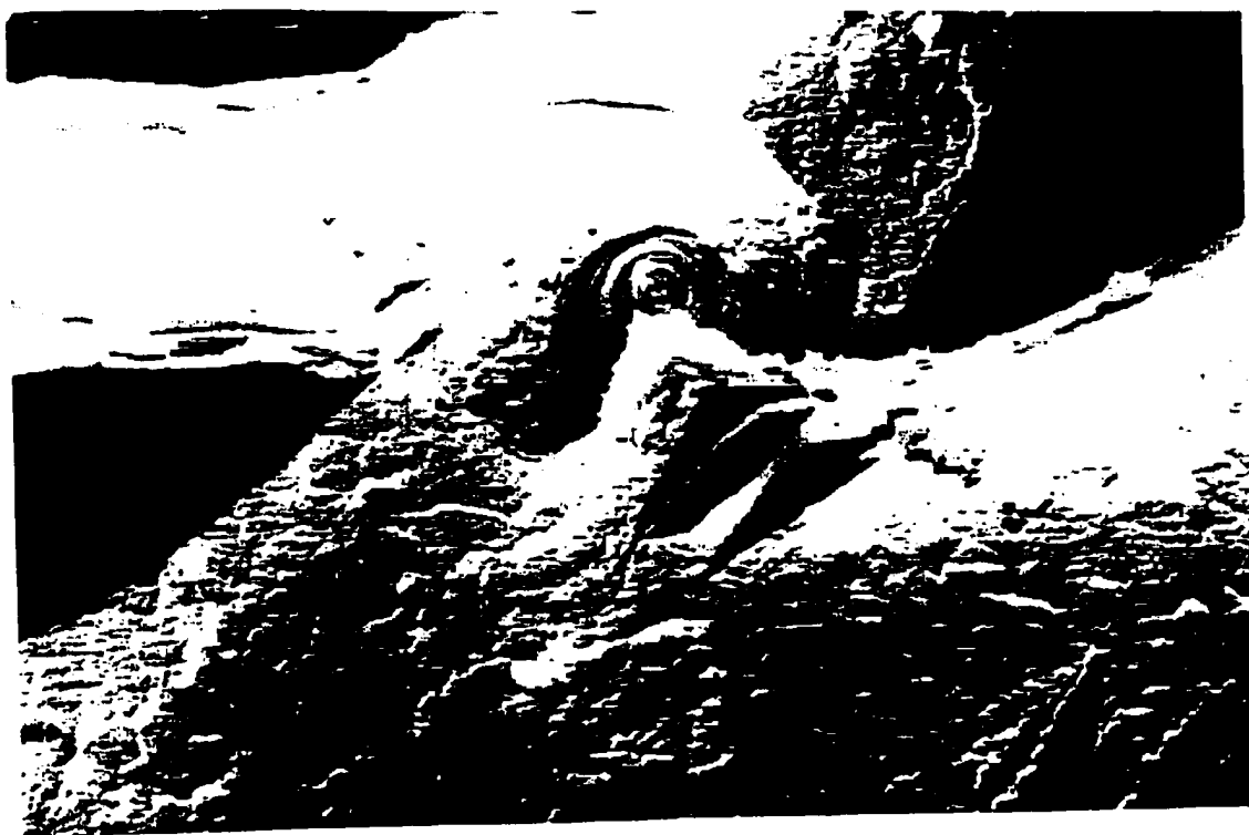
Figure 3. Transmission electron photomicrograph of low cationic/nonionic liposomal shampoo composition upon accelerating aging at 50°C for 4 weeks at a magnification of 80,000X.
