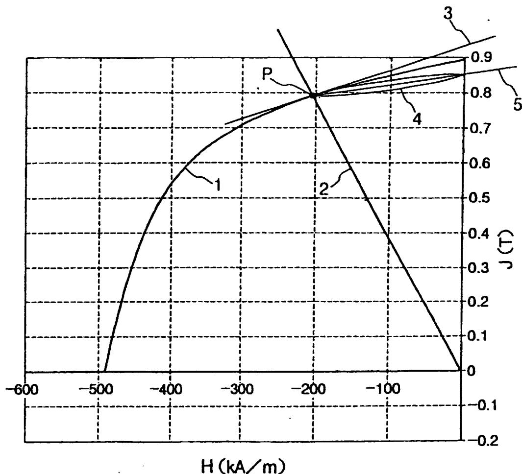
No.1: Demagnetization Curve
