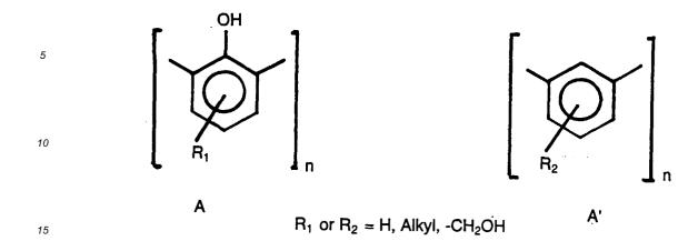
[0016] A typical convenient resin is for instance a phenyl aralkyl resin in which R<sub>1</sub> is -CH<sub>2</sub>-φ- having a basic structure of alternated moieties A/A'. A variety of such resins are sold under the generic name of ®Xylok by Mitsui Toatsu Chemical. Japan.
