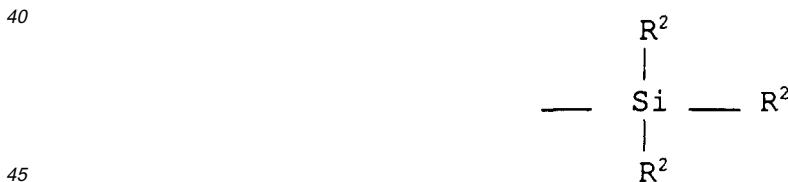
where  $\text{R}^2$  is an alkoxy of 2 to 4 carbon atoms, with 2 carbon atoms being particularly preferred; Alk is a divalent hydrocarbon of 2 to 4 carbon atoms, with 3 carbon atoms being particularly preferred; and n is an integer of from 3 to 5, with 4 being particularly preferred.
