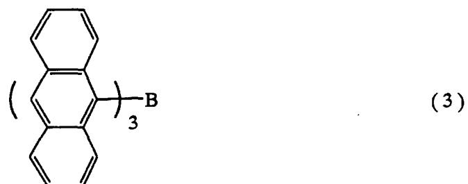
**[0018]** The compound represented by the formula (3) is one of the borane derivatives of the above formula (1) wherein  $n$  is 3,  $R_1$  to  $R_6$  are each hydrogen atom, and  $Z_1$  and  $Z_2$  are benzo-condensed.
