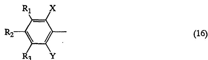
40 wherein R<sub>1</sub> to R<sub>3</sub> are each independently a hydrogen atom, a saturated or unsaturated hydrocarbon group, an aromatic group, a heterocyclic group, a substituted amino group, a substituted boryl group, an alkoxy group or an aryloxy group; and X and Y are each independently a saturated or unsaturated hydrocarbon group, an aromatic group, a heterocyclic group, a substituted amino group, an alkoxy group or an aryloxy group; and
