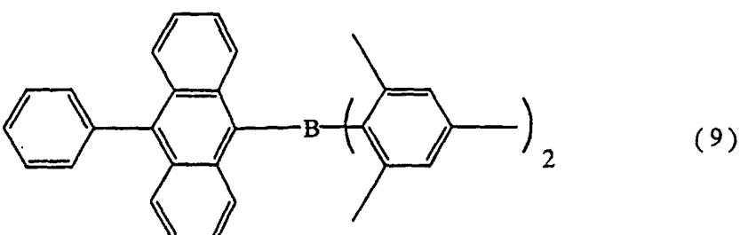
[0024] The compound represented by the formula (9) is one of the borane derivatives of the above formula (1) wherein n is 1, R<sub>1</sub> and R<sub>3</sub> to R<sub>7</sub> are each hydrogen atom, R<sub>2</sub>, X and Y are each methyl group, R<sub>8</sub> is a phenyl group, and Z<sub>1</sub> and Z<sub>2</sub> are benzo-condensed.
