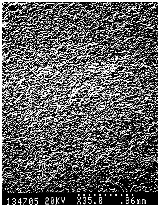
FIGURE 3 SEM photomicrograph of polypropylene-coated EBS paper. 35X magnification.
