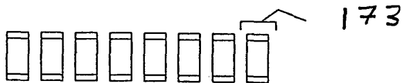
F I G . 1 7 C CROSS SECTION OF THE THERMOMATERIAL CHIPS WITH THE LAYERS FOR SOLDERING.
