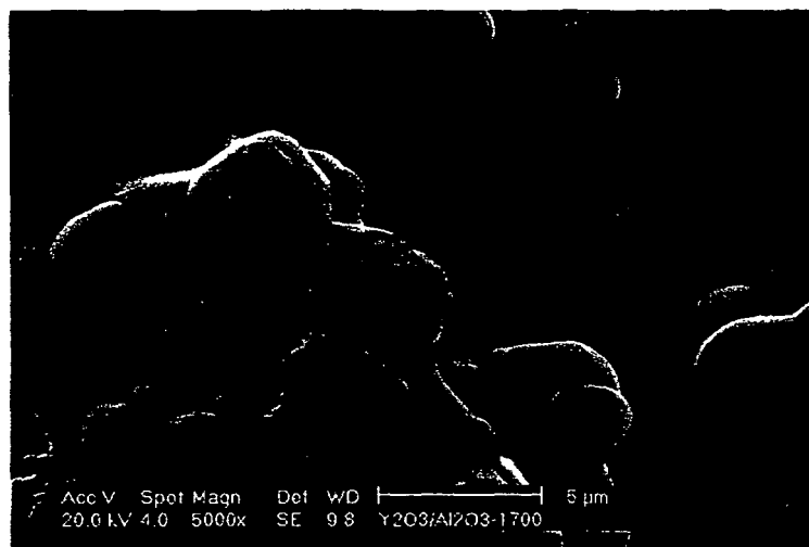
Surface of 1700°C×3h Co-sintered product (×5000)
