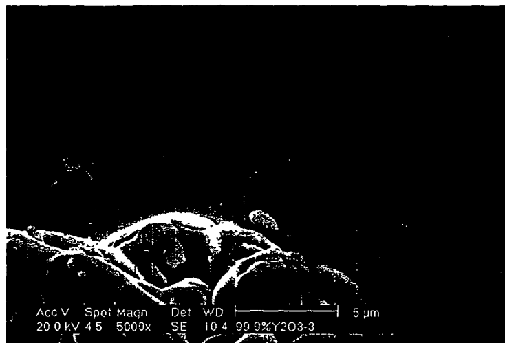
Surface of 99.9% Y_2O_3 sprayed product ( \times 5000 )
