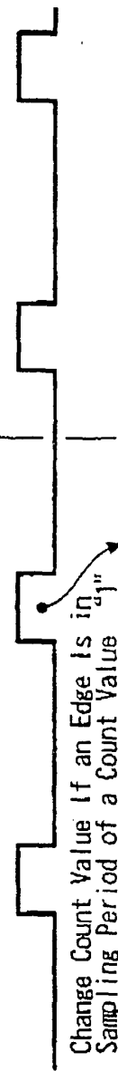
FIG. 2D Detection Pulse for Detecting Presence or Absence of Edge in Sampling Period
