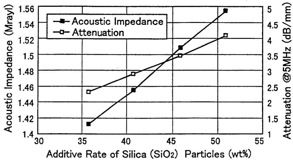
Relationships between Additive Rate of Silica (SiO<sub>2</sub>) Particles and Acoustic Impedance, and Attenuation
