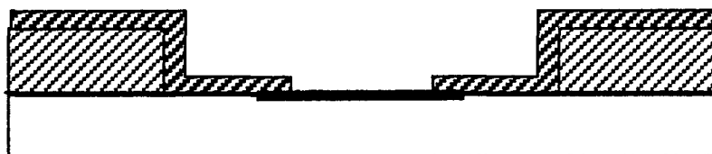
FIG. 2(E) ETCHING, FINISH
