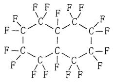
[0120] In the seventh embodiment, since perfluorodecalin contains no hydrogen atom, the resulting interlayer insulating film is a fluorinated amorphous carbon film containing only carbon and fluorine atoms. The fluorinated amorphous carbon film had a dielectric constant of 2.3 immediately after deposition.
