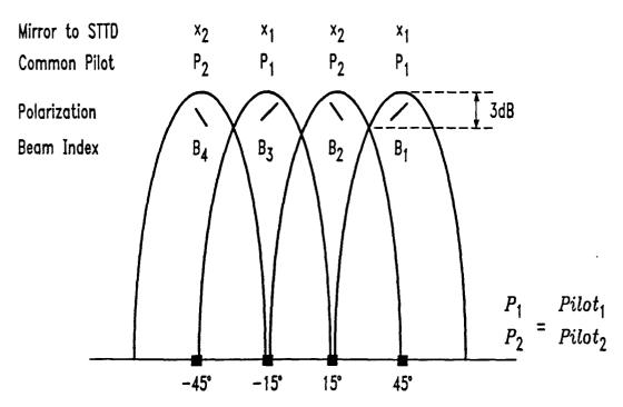
Combine space—time block code to switch beams.
