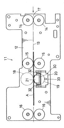
1... Magnetic Card Reader 71... Magnetic Head 82... Support Shaft 20
