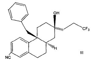
(h) reacting the compound of formula **III** so formed with aqueous sodium hydroxide in a polar protic solvent to form the compound of formula **II**
