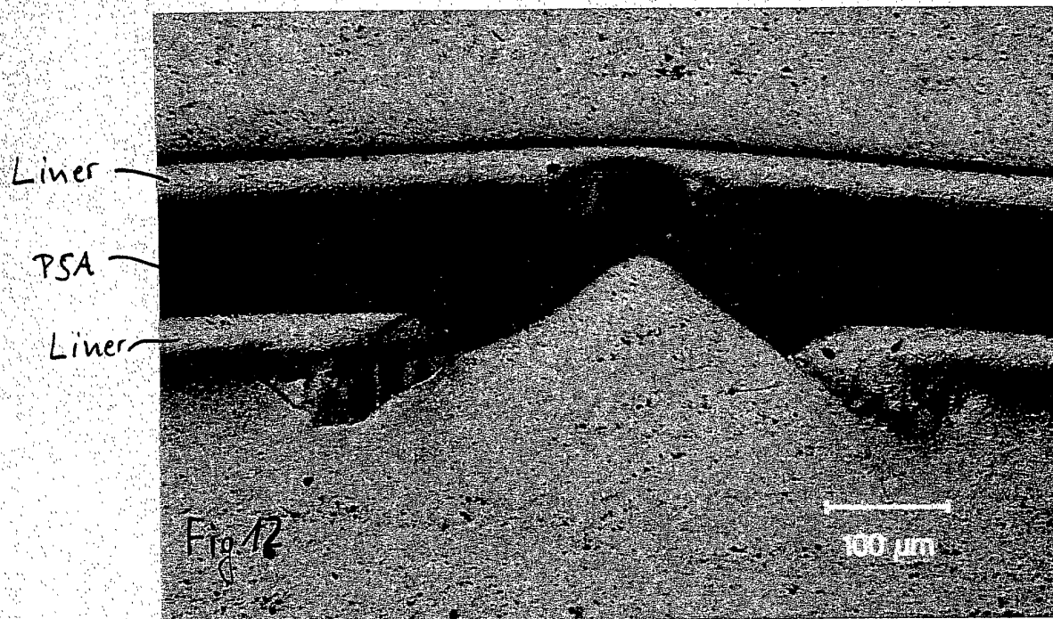
60% of 50 watt laser (Rofin-Sinar), 5 kHz, 300 mm/sec. cutting speed
