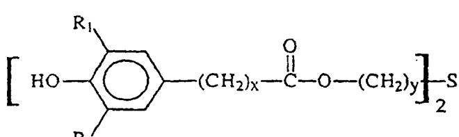
wherein, in the formulae (I) - (IV) above, R<sub>1</sub>, R<sub>2</sub>, and R<sub>3</sub> are the same or different alkyl groups having 3-9 carbon atoms and x and y are integers from 1 to 4.
