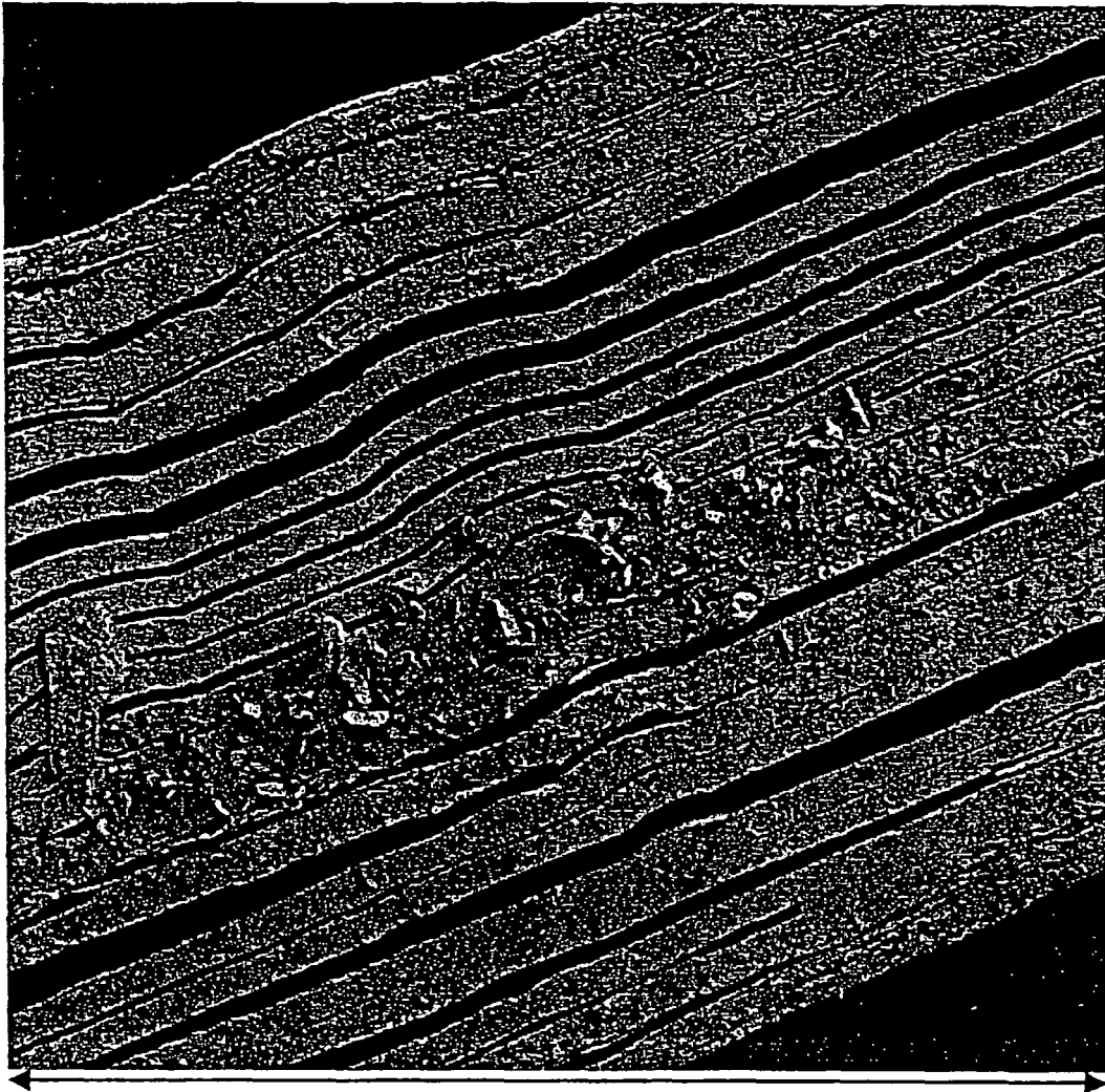
Fig. 2B A Typical Example of Delineation of Preferred Failure Planes from the Slot Test (Example 4)
